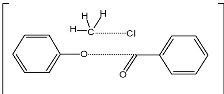
Intermediate inside the zeolite cavity
